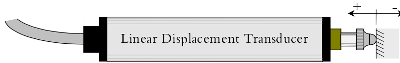
Figure 4.11 General description of a Linear Displacement Transducer (LDT). Positive values of the displacement are obtained when the point of the LDT is going inward and negative values when going outwards.
